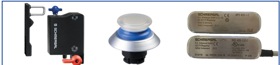
Examples of machine controls designed for hygienic applications. They feature smooth surfaces and transitions, IP69K rating, and/or ECOLAB approved materials. Other considerations include use of stainless steel or blue colored components that are easily identifiable if they fall into food lines.
