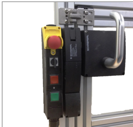
Picture 2: machine controls with emergency stop, mounted at a safety guard access door.
