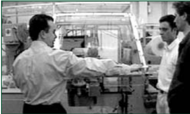
This movable guard permits access to load and unload material and clear jams.
