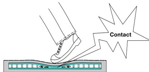
The safety mat consists of two separate current-carrying steel plates. The plates are held apart by insulating strips. Upon actuation of the pressure-sensitive safety mat, an electrical cross-wire short is produced between the steel plates. The connected safety-monitoring module evaluates this signal and stops the hazardous movement.
