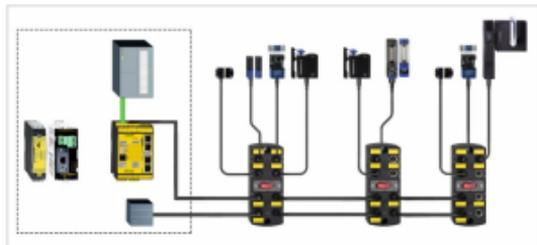
The electronic safety devices also have an option for serial diagnostics. Instead of a basic PNP output, a serial data package will send detailed information of an individual switch. This information can be communicated via a wide range of network protocols by the use of a Gateway and be displayed on a machines' HMI.
