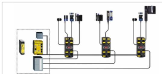
Schmersal electronic safety devices will feature an auxiliary PNP semiconductor output to provide basic information of the guard status. In order to preserve the individual switch status in a series or zoned connection, Schmersal offers both passive and active field-box options.
