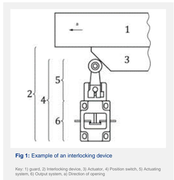
Fig 1: Example of an interlocking device
