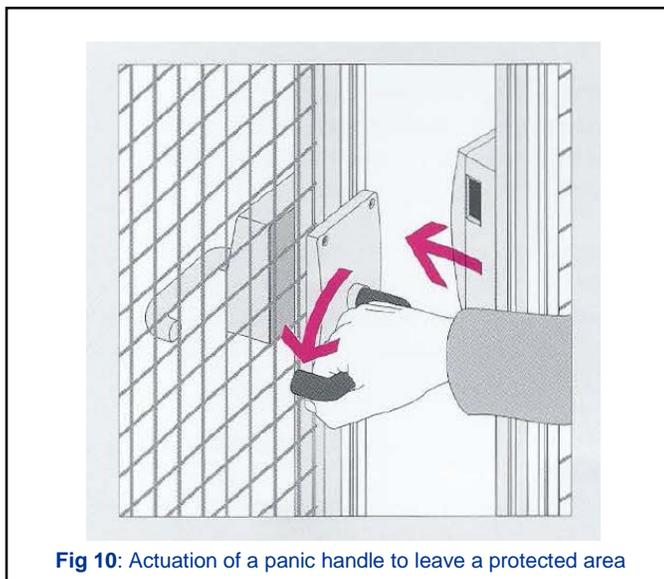
Fig 10: Actuation of a panic handle to leave a protected area
