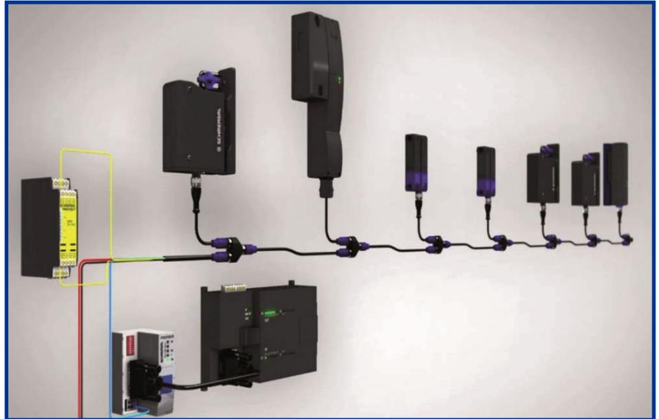
Image 1: Serial Diagnostic devices wired in series, to gateway to network Bus
