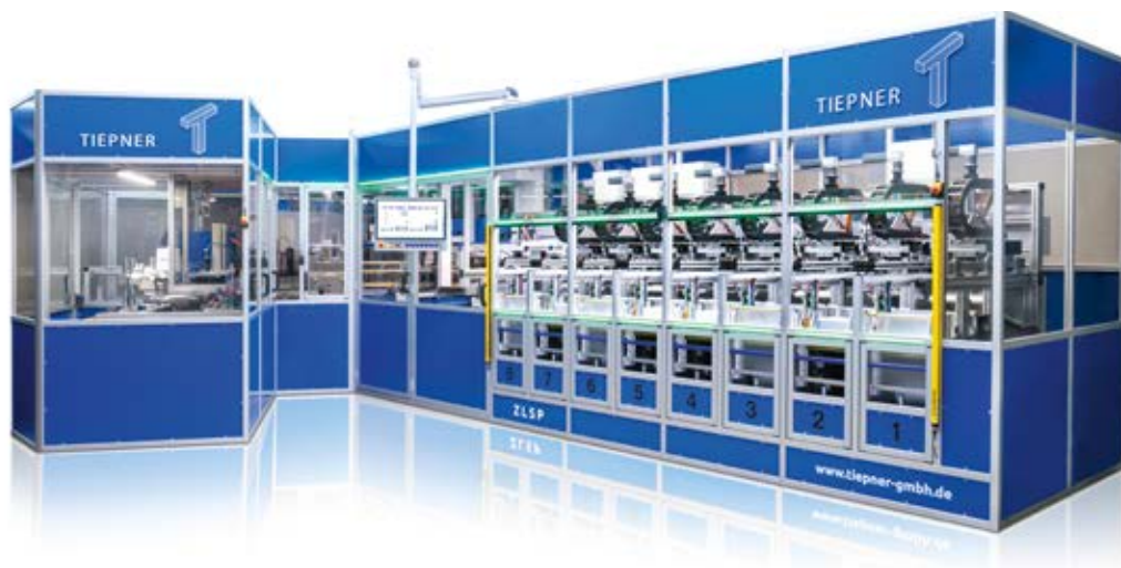
Fig. 7: As a specialist in the production of plastic cards, Tiepner also designs and builds more complex systems that take over upstream process steps such as the production of the laminate, which consists of up to eight layers.
