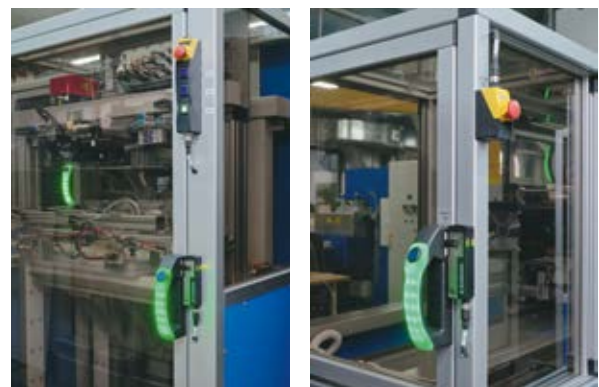
Fig. 4 left: A separate control panel from Schmersal's BDF 100 series is used for additional operating functions (top in picture).
