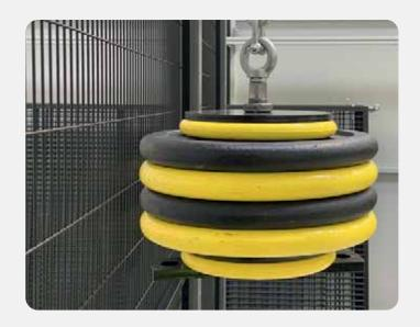
Mass release height from the ground (mass load center): h0 = 3,060 mMass impact height from the ground (mass load center): h1 = 1,420 m $\Delta H = h0 - h1 = 3,06 - 1,42 = 1,64 \text{ m}$
