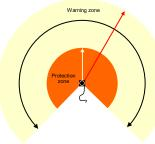
270 degree detection angle 5 meter protection zone 20 meter warning zone
