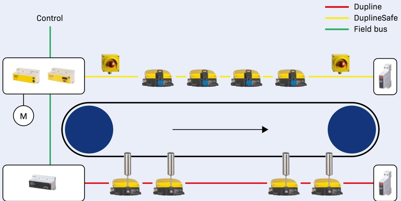
Circuit diagram for networking of pull-wire emergency stop switches with DuplineSafe or belt misalignment switches. Data exchange with the higher-level control takes place via a standard field bus (Profibus DP, etc.).
