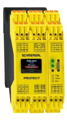
Four different programs are available. Each program can be precisely adapted – without any programming knowledge, simply with the menu and clear text messages – to the specific application case. The drop-out delay and the debounce times can be set individually, and numerous parameters such as the short-circuit monitoring can be set as required – a definite advantage in comparison with safety relay modules.
