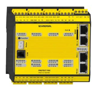
The safety control system PSC1 consists of freely programmable compact safety controllers with I/O extension modules for signal processing of EMERGENCY STOP switches, guard door switches, light grids and other mechanical and electronic safety switchgear. Additionally there is the possibility via numerous functions to monitor axes. Using the universal communications interface, a connection can be established to all the standard field bus systems.
