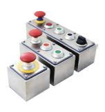
The NBGLC is a IP69 rated stainless steel enclosure for pushbuttons designed for hygienic applications, designed in accordance to DIN EN 1672-2 with hygienic and chemical-resistant materials. The enclosures are constructed from stainless steel 1.4301 (X5CrNi18-10), AISI 304, (V2A). Silicone seals are provided to fill the gaps for screws, faceplate, and base to achieve IP69 rating for wash downs. These seals are blue to be easily detectable by vision systems.
