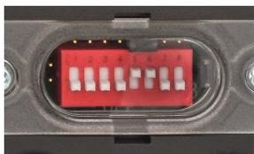
Dipswitches for configurations based on wiring schemes
