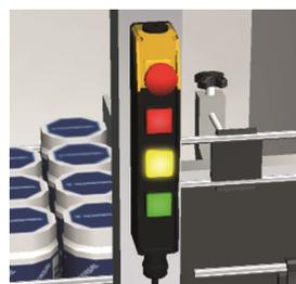
**BDF200** - designed to offer various machine or process controls conveniently located at the guard door in a housing that matches the AZM201. Each control station can include operators in up to 4 positions which can be configured (and field labeled) to user-defined application needs including an integrated Emergency Stop palm button.
