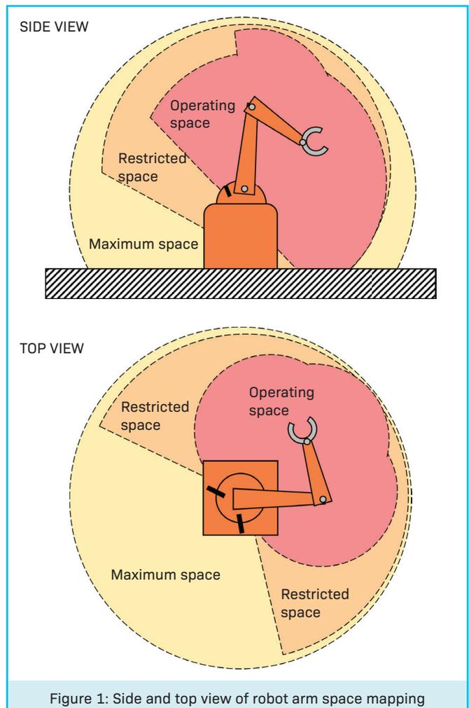
Figure 1: Side and top view of robot arm space mapping
