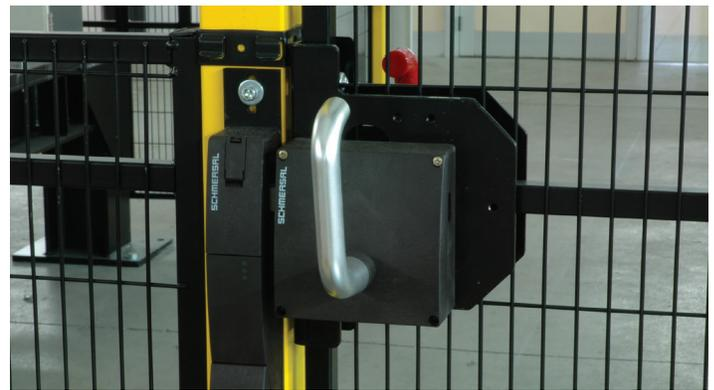
This door lock has an emergency release handle inside the robot cell.
