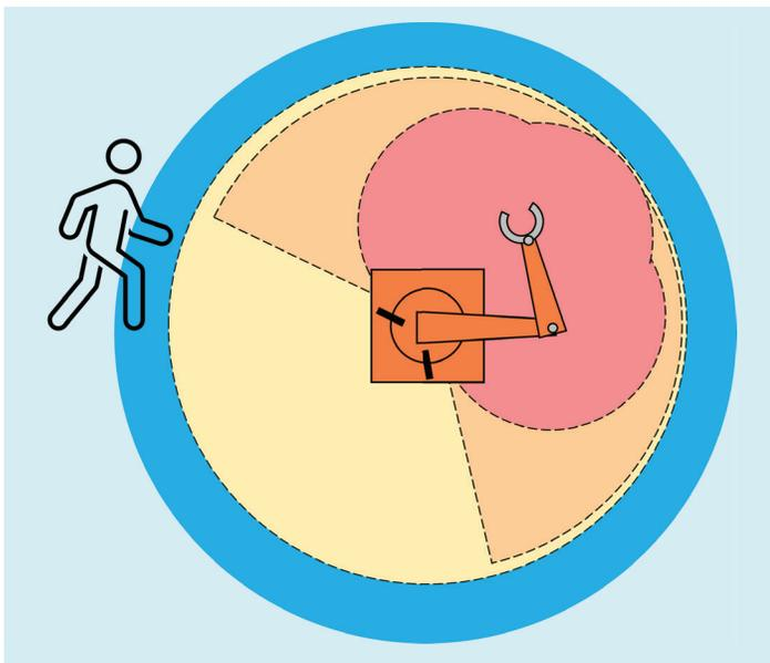
Many applications become ineligible because the calculated minimum safe distance for placing these devices is impractical. Traditional industrial robotics applications which consist of large payloads and high speeds generally have longer stoppage time and may need a greater distance than is feasible.
