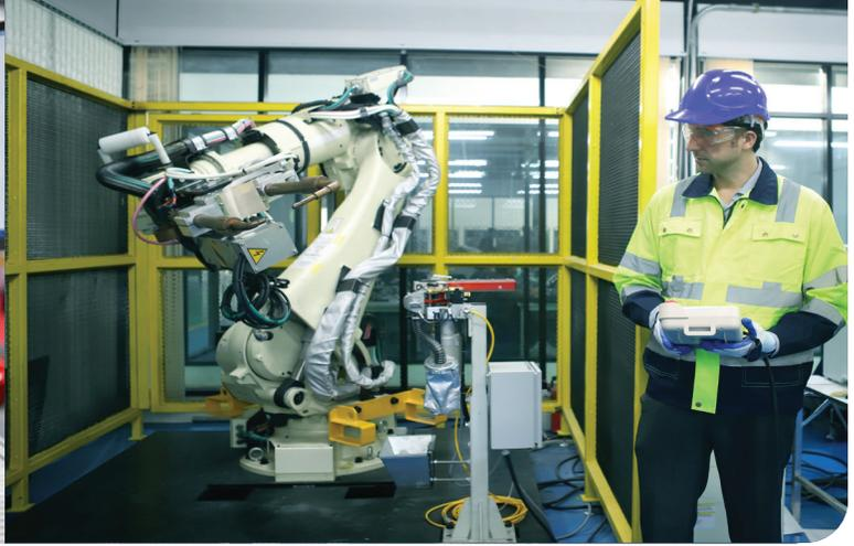
Robots offer a means to simplify and improve efficiency with a process and can complete tasks that pose too great of a hazard to be handled by human operators. This, however, does not remove all hazards from a machine or process, yet it creates new unique hazards which must be guarded to protect personnel while working directly or around the robot.
