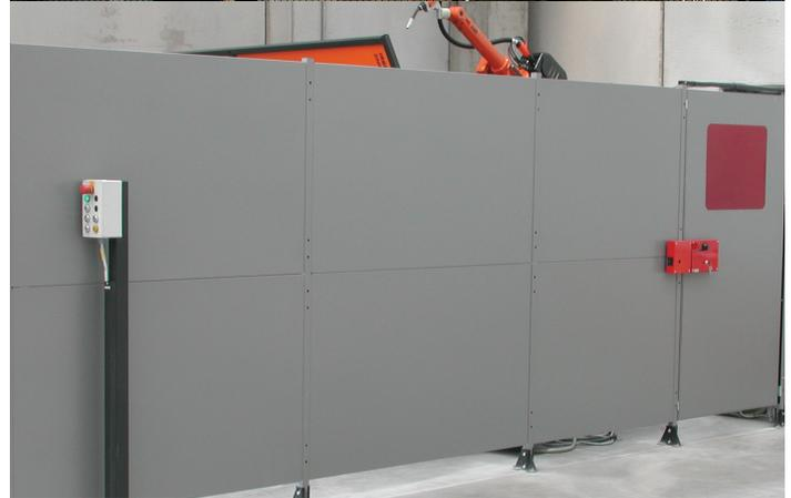
Top: safety fencing provides a good view of the robot cell
