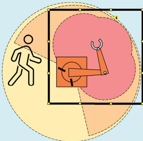
Here the physical barrier has been placed outside the maximum space, restricting access to the hazardous area.
