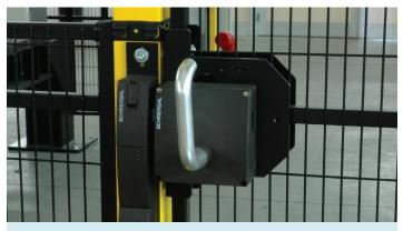
This door lock has an emergency release handle inside the robot cell.
