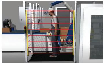
Animation of a double reset. The second pushbutton is mounted outside the cell. The process includes interupting the light curtain.
