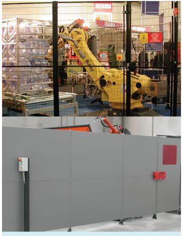
Top: safety fencing provides a good view of the robot cell Bottom: A robot cell with a opaque barrier.
