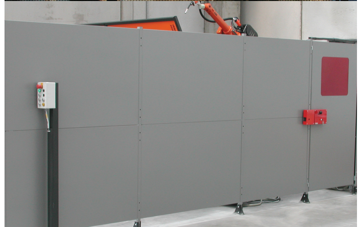
Top: safety fencing provides a good view of the robot cell Bottom: A robot cell with a opaque barrier.
