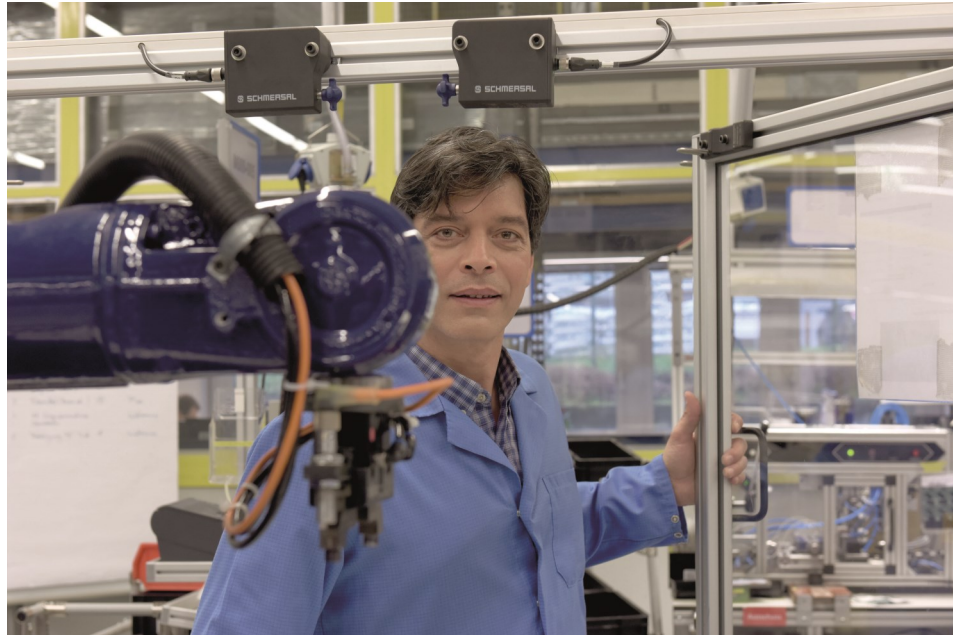
Image 1: worker enters a robot cell protected by a guard door with safety interlock switches.
