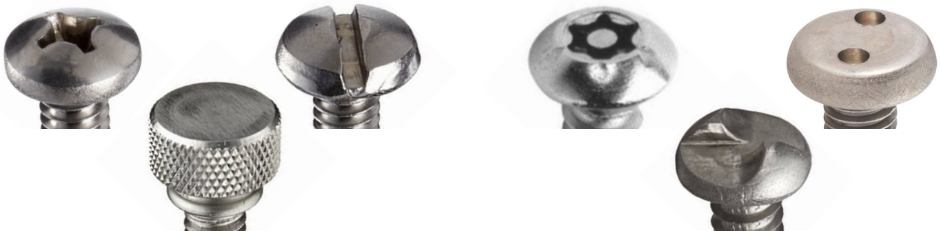
Image 2: examples of various fasteners. To the left: fasteners which do not require a special tool for removal. Slotted head and thumb screws can easily be removed and should not be used to secure fixed guarding. To the right: examples of tamperproof screws, which require special tools for removal and thus can be used to secure fixed guards. Tools which are considered not common to the operator is dependent on the specific factory site.
