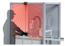
Detects access into critical zone at point of operation.
