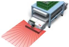
32 safety area patterns to accommodate the AGV travel path for collision protection
