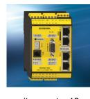
The safety control system PSC1 is a modular and freely programmable compact safety controller with I/O extension modules for signal processing of emergency stop switches, guard door switches, light grids and additional mechanical and electronic safety switchgear. Additionally, there is the possibility via numerous functions to the safe speed Using the universal
