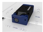
Actuator alignment tolerances: Hole dia. is 8 mm wider than bolt 1 mm - 7 mm offset from switch
