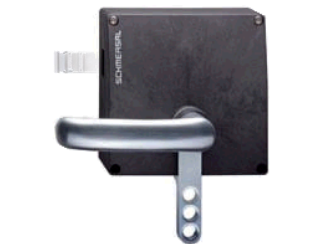
Optional integrated lockout device on door handle is one of three methods for lockout. Actuator retracts into door handle housing when opened (handle is horizontal)
